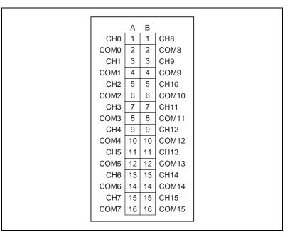
Figure 1-1. Front Connector Pinout Assignments
