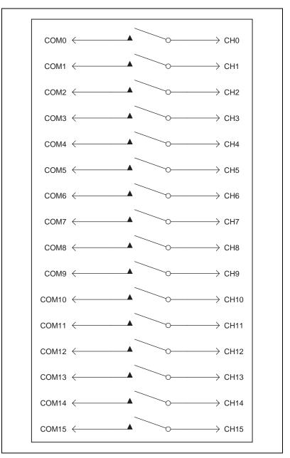
Figure C-1. NI 2565 Switch Architecture
