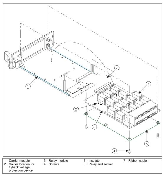
Figure B-1. NI 2565 Parts Locator Diagram
