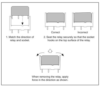
Figure B-2. Replacing a Relay
