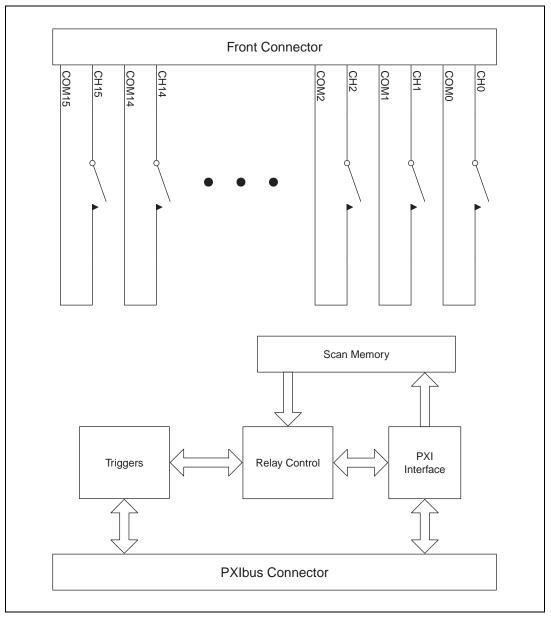
Figure 2-1. NI 2565 Module Block Diagram
